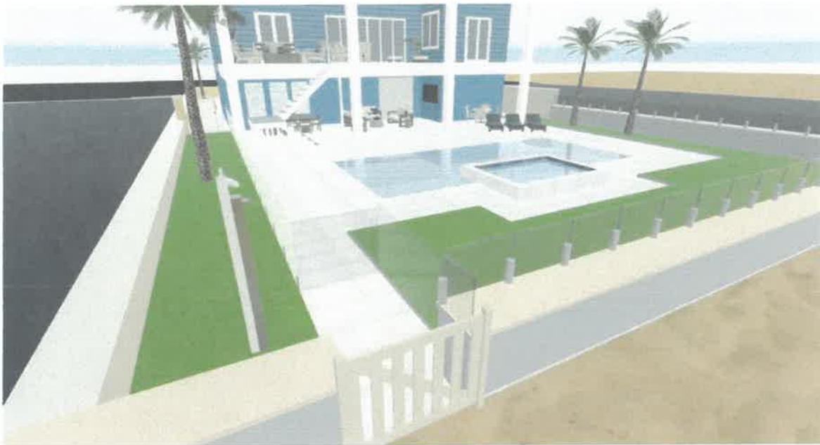
Exhibit A-3: Full property overview from the Northwest: pool (Central), inner 4' glass fence - Left side of pool deck (North), seawall/retaining wall with glass topper – Bottom section(West), side-wall with glass topper – right side(South), and beach access
