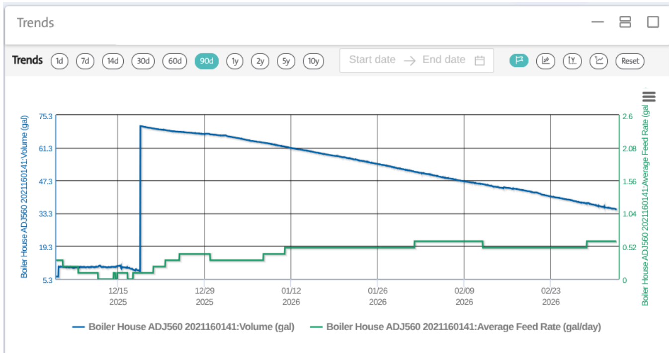
Figure 3. Insight data trend showing tank level and usage rate
