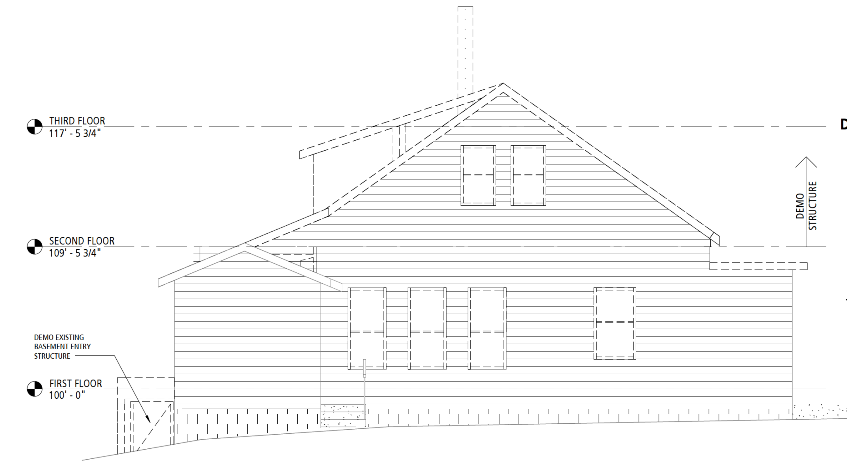
11 OVERALL EAST BUILDING ELEVATION - DEMO 1/4" = 1'-0" 23 / A100
