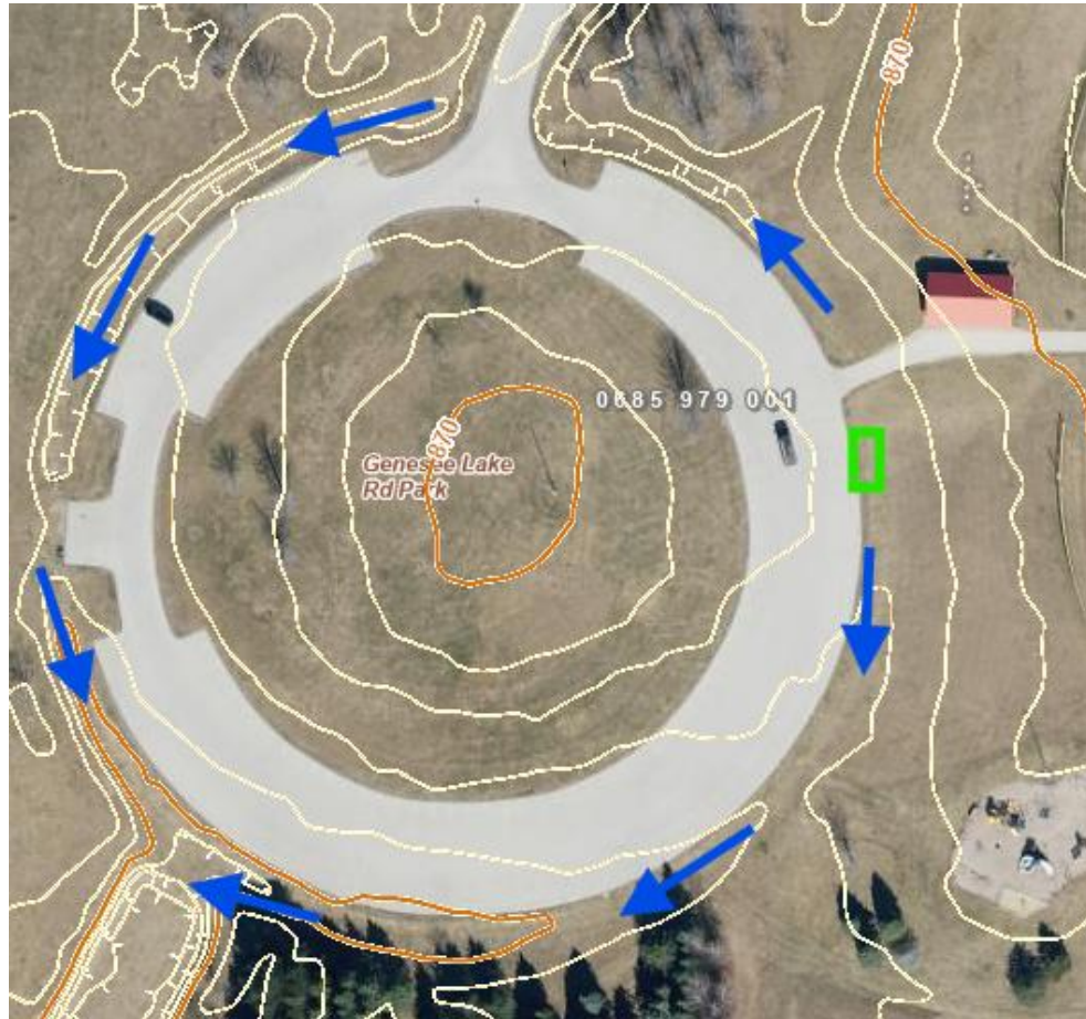
Topography of circular parking lot depicting stormwater flow and high point at asphalt path. Proposed enclosure location highlighted in green.
