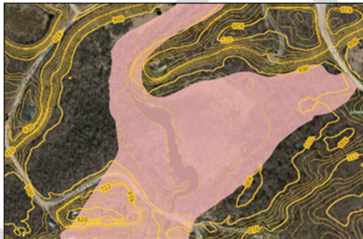
Figure 8. The Mapped Floodplain May Not Always Align with On-the-Ground Contour Elevations
