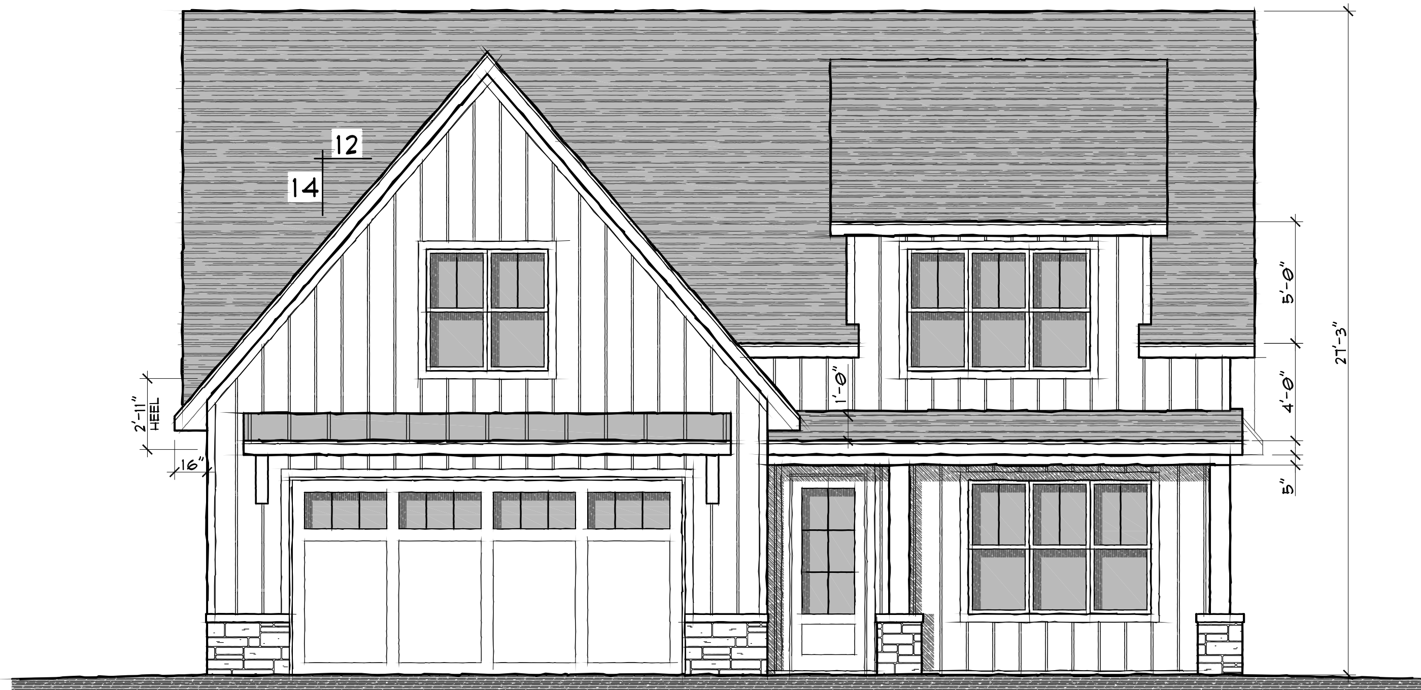
FRONT ELEVATION SCALE: 1/4" = 1'-0"
